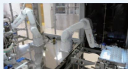
Filling equipment featuring robotics technology
